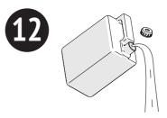
Monitor the fullness level of the drain tank that the liquid is to flow into. When full, empty the tank.
