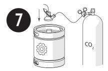
Ensure that the gas cylinder reducing valve is set at a pressure of 1 bar (15 psi).
