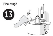
Clean the flask drain channel with the mini brush, then wipe the drain hole with a sponge dipped in warm water with a mild detergent. Rinse with hot water.
