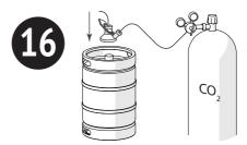
In order to maintain cleanliness, do not drain water used for flushing at the last treatment stage from the beverage supply line until subsequent use of the dispenser. Connect the intake head removed from the flush keg to the beverage keg.
