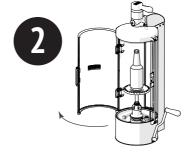
Open the protective door and place an empty small volume flush tank on the tray, having adjusted the adjusting assembly to its height.
