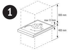
Ensure that the installation location matches the dimensions specified in the picture and indicated on the template. Fix the template and use it to make markings on the table board.
