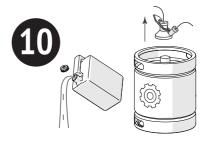
Disconnect the intake head from the flush keg without dismantling the gas and beverage supply channel hoses. Empty the drain tank.
