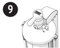
Before releasing the bottle slightly open the drain channel by turning the flow control valve counterclockwise. The pressure in the beverage container takes approximately 10 s to even out with atmospheric pressure.
