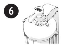
Turning the flow control valve within one rotation, choose the filling speed based on the foam formation intensity.
