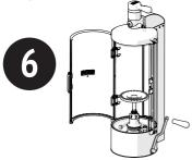
Screw the bottle tray on the end of the shaft with a backing plate on it as well as the handles to the appropriate locations.
