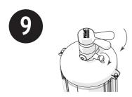
After the performance time of the treatment stage expires, shut off the beverage supply channel and then shut off the drain channel.
