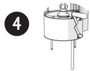
Place the dispenser on the counter top by aligning it with the pre-drilled holes. Insert power cord through rear hole.
