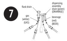
Connect the gas, beverage supply, and drain hoses (flask and dispensing assembly) with the appropriate dispenser tubes using JG-connections included in a standard set
