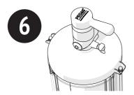
Ensure that the switch handle is in the neutral position.
