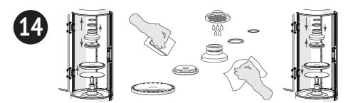
Remove the backing plate from the bottle tray. Twist off the pouring head bushing, detach the gasket, remove the seal from the groove, and remove the gasket from the hole. Wipe the removed components with a sponge dipped in warm water with a mild detergent.
