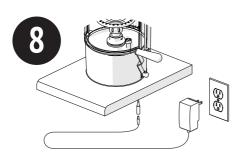
Connect the power adapter to the appropriate device connector under the table board.
