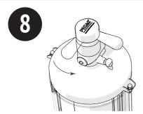
Once you have reached your desired fill line, shut off the beverage supply channel by positioning the switch handle into the neutral position and the beverage supply will stop.
