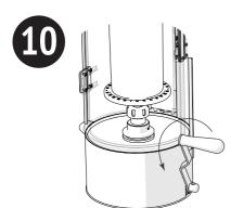
Lower the full beverage container by turning the adjusting assembly knob counterclockwise until it stops, then open the protective door of the dispenser.
