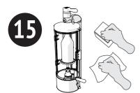
Wipe the inside surface of the flask with a sponge dipped in warm water with a mild detergent. Then wipe the inside and outside surfaces of the flask with a clean wet cloth. Wipe the flask thoroughly inside and outside with a clean lint-free cloth until dry.
