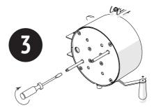
Use a screwdriver to screw studs into the threaded holes in the bottom of the dispenser.
