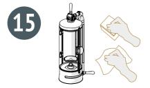
Wipe the inside surface of the flask with a sponge dipped in warm water with a mild detergent. Then wipe the inside and outside surfaces of the flask with a clean wet cloth. Wipe the flask thoroughly inside and outside with a clean lint-free cloth until dry.
