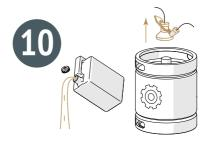
Disconnect the intake head from the flush keg without dismantling the gas and beverage supply channel hoses. Empty the drain tank.
