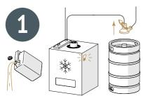
Disconnect the beverage keg from the dispenser and turn off your glycol system if possible. Empty the drain tank.
