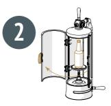
Open the protective door and place an empty small volume flush tank on the tray, having adjusted the adjusting assembly to its height.
